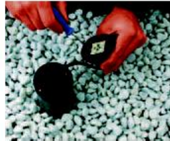
Step 3 Insert the LED module into the inner casing and screw in place.
