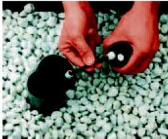
Step 1 Insert the supply cable H05RN-F 2 x 1 mm 2 into the inner casing through the outer casing and the PG-7 cable penetration.
