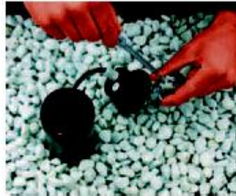
Step 2 Connect the supply cable to the terminals on the back of the LED module.
